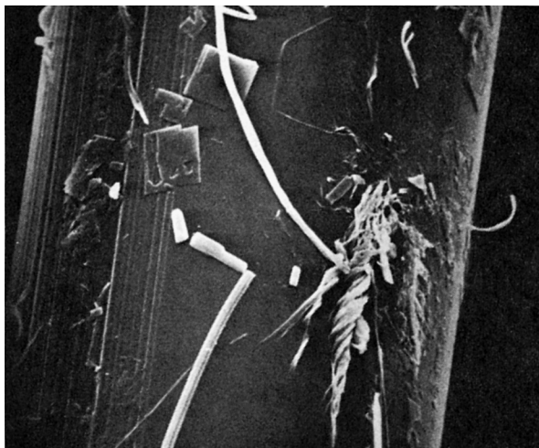
Fig. 21. Additional crystal forms grown on nylon 6 filament exposed to pentanol vapor ( \times 1300 ).
